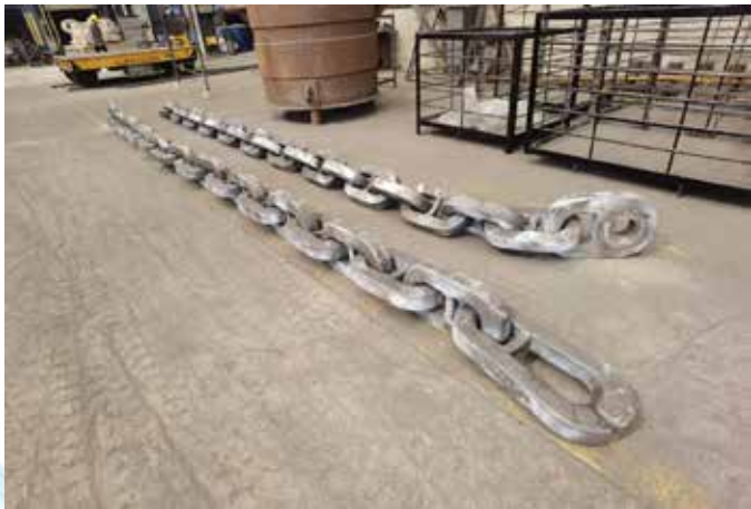
Mining Dragline Chains Developed and Manufactured Using Precision Shell Special Technology
