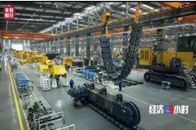
Development and Manufacture of a Four-Wheel and One-Track Product for China's First 700-ton Hydraulic Excavator
